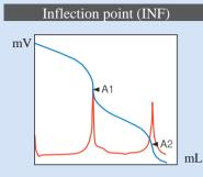
Results are calculated by inflection points detected from the shape of titration curve using tangential lines of the curve.
