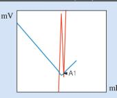
An end point is decided by changing slope of straight lines along the waveform. Titration curve looks V-shape. End point is the first intersection of the two lines.
