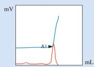
An end point is decided by changing slope of straight lines along the waveform. End point is the first intersection of the two straight lines.
