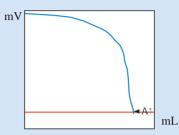
End points are set to fixed potentials or pH. When the value approaches to the set points, titrant injection volume is controlled precisely for accurate measurement.
