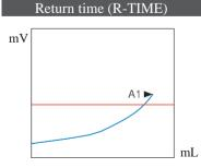
End point is decided by a set time. Titration ends after keeping a reference potential or pH value for the time.
