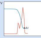
An end point is decided by changing slope of the straight lines. When the slope becomes flat, intersection of the two lines is end point. The second intersection is the end point.
