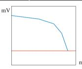
Control the potential or pH by titration to reach a reference value. e.g.) Using for pH control before
