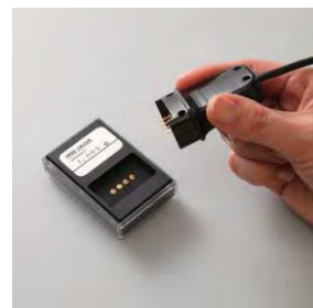
● Check the probe by probe checker.
